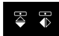
Left: mirror end to end button. Right: mirror side to side button.
